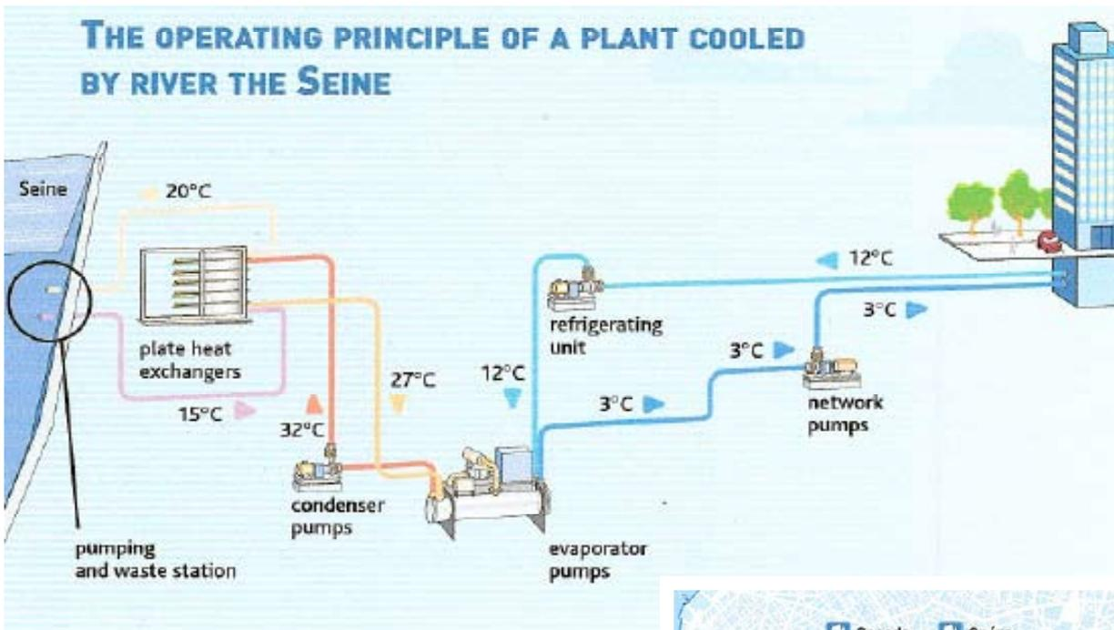
Schematic sketch of a district cooling plant cooled by Seine river water.
