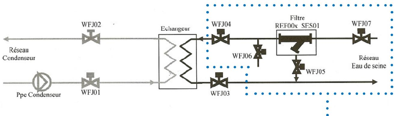
Heat exchangers with protecting cooling water filters. The Y-strainer has been replaced with a Bernoulli BSS 250.
